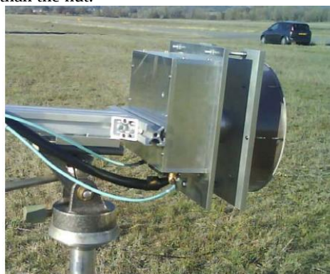
Figure. 3 Sensor (planar folded that reflect array antenna)
